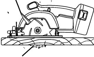
**BLADE EXPOSED ON UNDERSIDE OF WORKPIECE**
